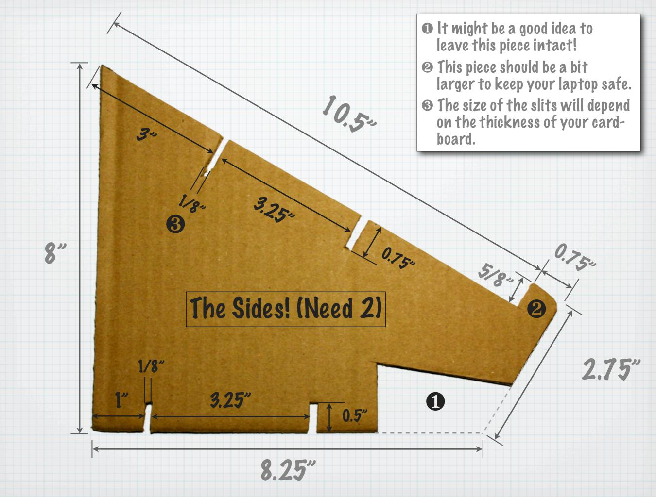
\*The dimensions of the two pieces are the same, the only difference is the orientation of the center slit.
